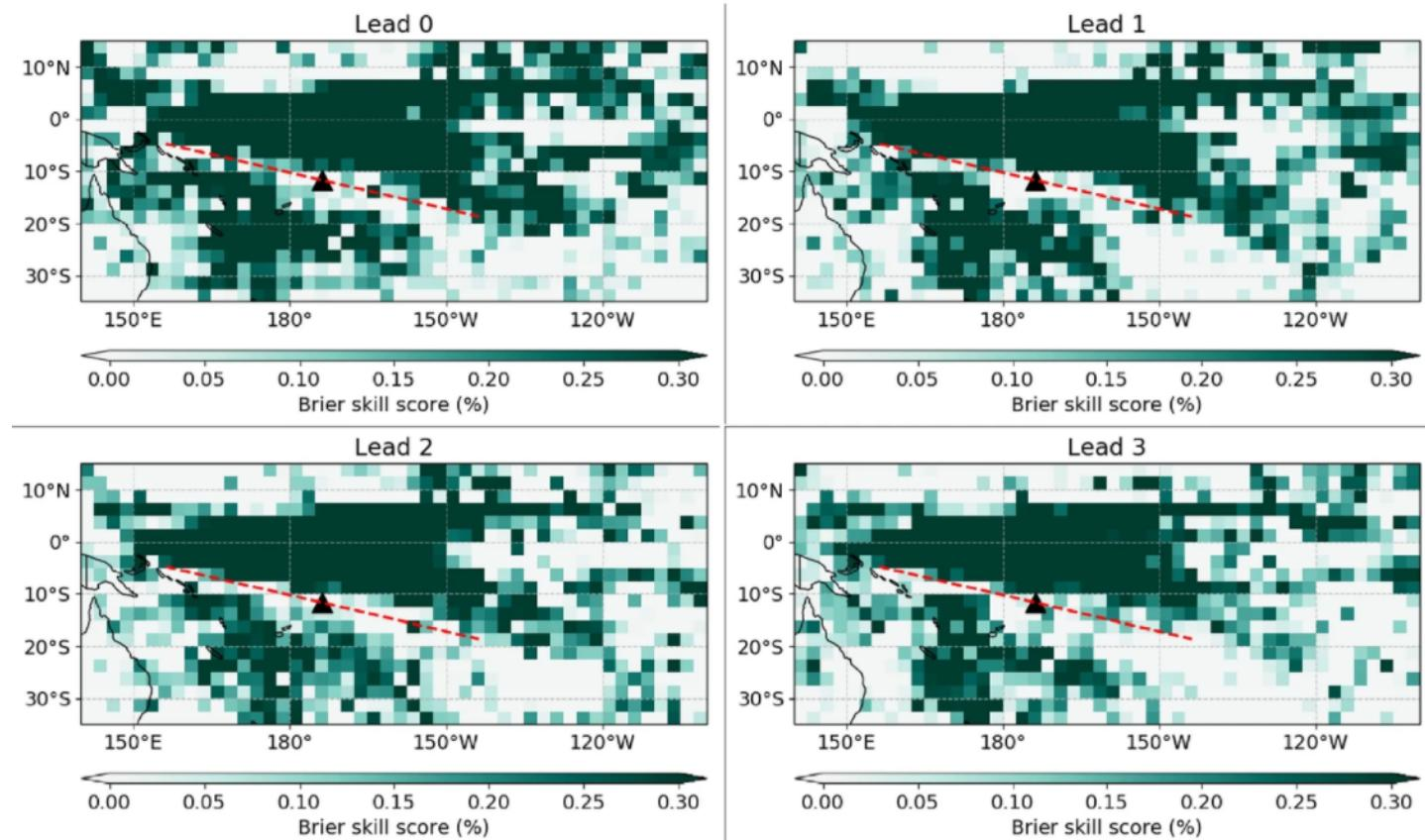
ACCESS-S1 precipitation verification skill scores for **a** weighted percent correct (WPC) and **b** Brier skill score for DJF months with 0–3 month lead times over the 1990–2012 hindcast period using GPCP as the observations dataset. The SPCZ and mean latitude is shown by the dotted red line and black triangle respectively, using GPCP data
